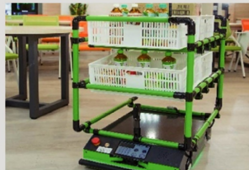
智慧商務 - 物流無人搬運車模擬教室 Intelligent Commerce Laboratory : Automated Guided Vehicle (AGV) Simulation Classroom
